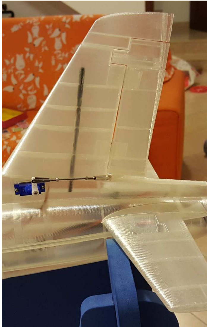
Carbon tube diameter 4 mm also for the rudder section.
