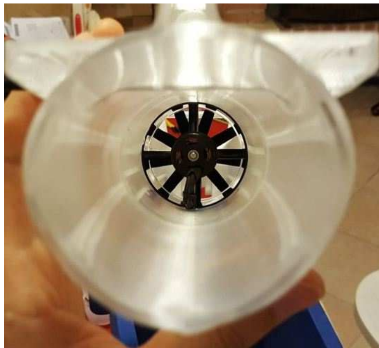
Detail of rear tube venturi (example with vemotec fan)
